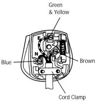
2. The wire coloured blue must be connected to the terminal "N" or coloured black.
